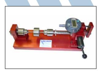
The *DIE CHECK* uses your standard plug gage sets with a dial or digital indicator to determine bearing lengths. Approach angles are also able to be calculated by taking two or more measurement on the angle. It's quick three step procedure, as shown on the left, makes it the perfect tool for the die shop or quality lab to insure that the die has a correct bearing length before going into production or problem solve after a die has failed.
