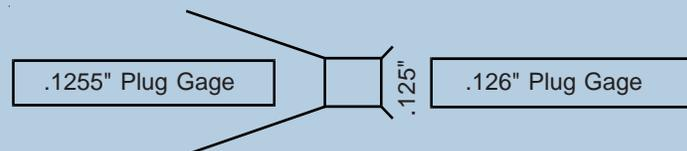
STEP 3 - Bring the plug gages into contact with the die and take the reading off the indicator which is the bearing length. To convert it into a percentage divide the reading by the dies diameter and multiply by 100.
