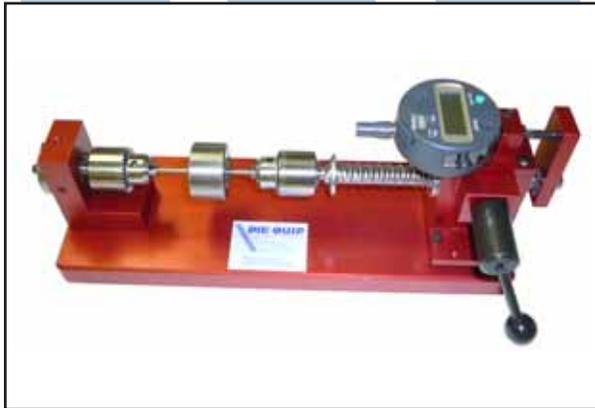
The *DIE CHECK* uses your standard plug gage sets with a dial or digital indicator to determine bearing lengths. Approach angles are also able to be calculated by taking two or more measurement on the angle. It's quick three step procedure, as shown on the left, makes it the perfect tool for the die shop or quality lab to insure that the die has a correct bearing length before going into production or problem solve after a die has failed.
