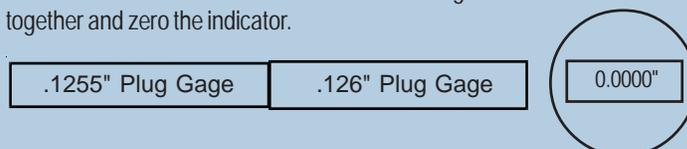
STEP 2 - Pull the plug gages back and insert the die.
