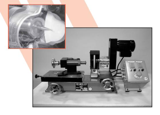
Our machine features accurate and repeatable angle settings with gage blocks. It is easy to operate and includes a diamond wheel dresser. We use standard ER20 collets which are available in 3/64 - 1/2" sizes (1.2 -12 mm). It also has adjustable depth stop and positive zero stop features and an optional vacuum system.
