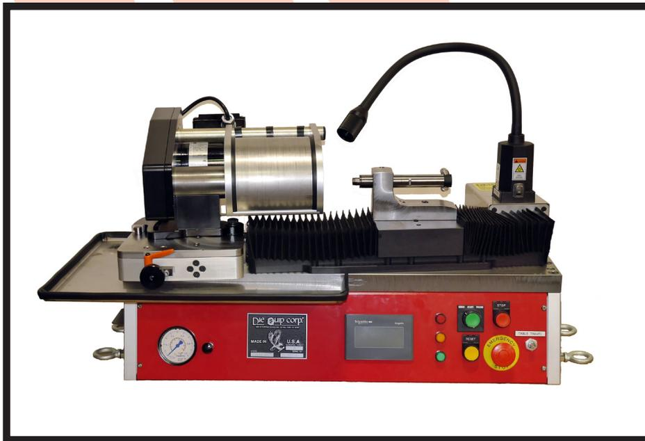
Our MGF is a semi-automatic grinding and polishing machine that has a powerful geared air spindle to reduce grinding times and reduce operator involvement compared to the HDF. This machine is designed to cut dies using the meeting point method or cutting dies to the next size. Its angle setting gage and zero stop makes it easy for any operator to produce accurate die geometry.
